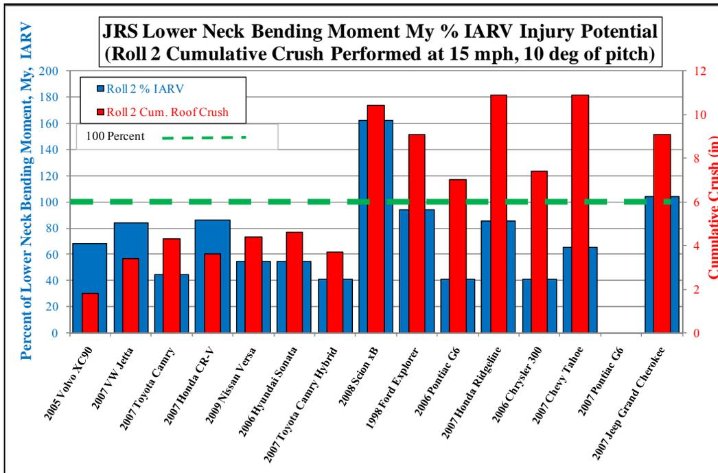
Figure 10. The relationship between cumulative residual crush in Roll 1 and 2 and the percent of lower neck bending moment relative to the IARV criteria
