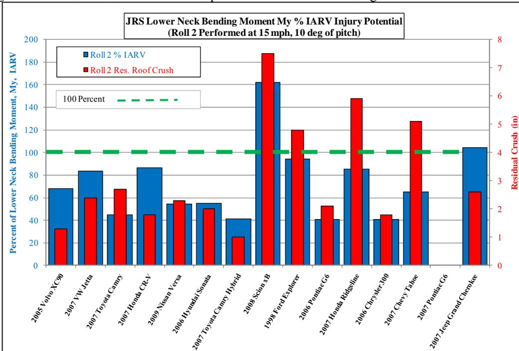
Figure 9. Residual crush in Roll 2 vs the percent of lower neck bending moment to the IARV criteria
