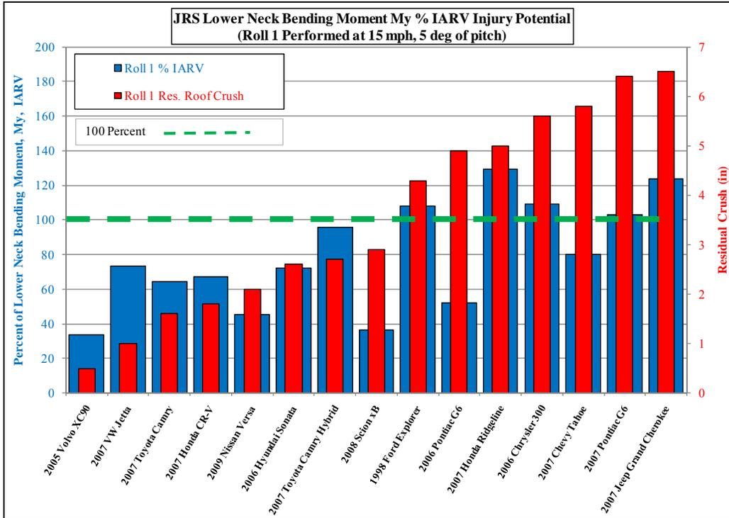
Figure 8. Residual crush in Roll 1 vs the percent of lower neck bending Moment to the IARV criteria
