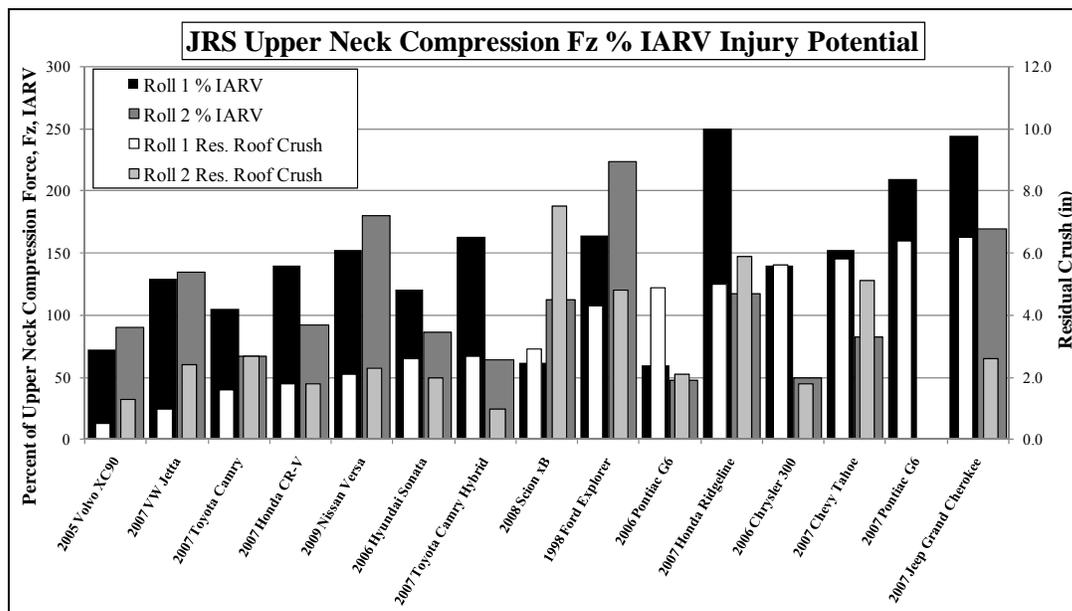
Figure 11. The relationship between upper neck compression force in each of two rolls expressed as a percent of the IARV criteria
