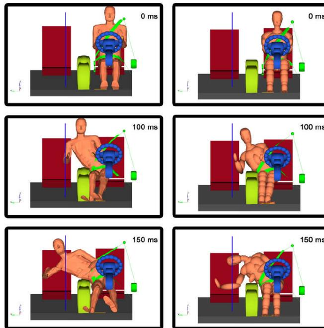
Figure 3. Illustration of the out-of-position extent of a far side dummy and human during yaw (100 ms) and trip (150 ms)
