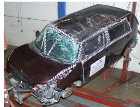
Figure 4: Vehicle Post Roll 2
