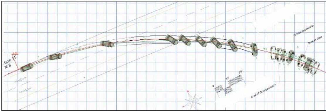
Figure 2. Typical rollover yaw trajectory by accident reconstruction
